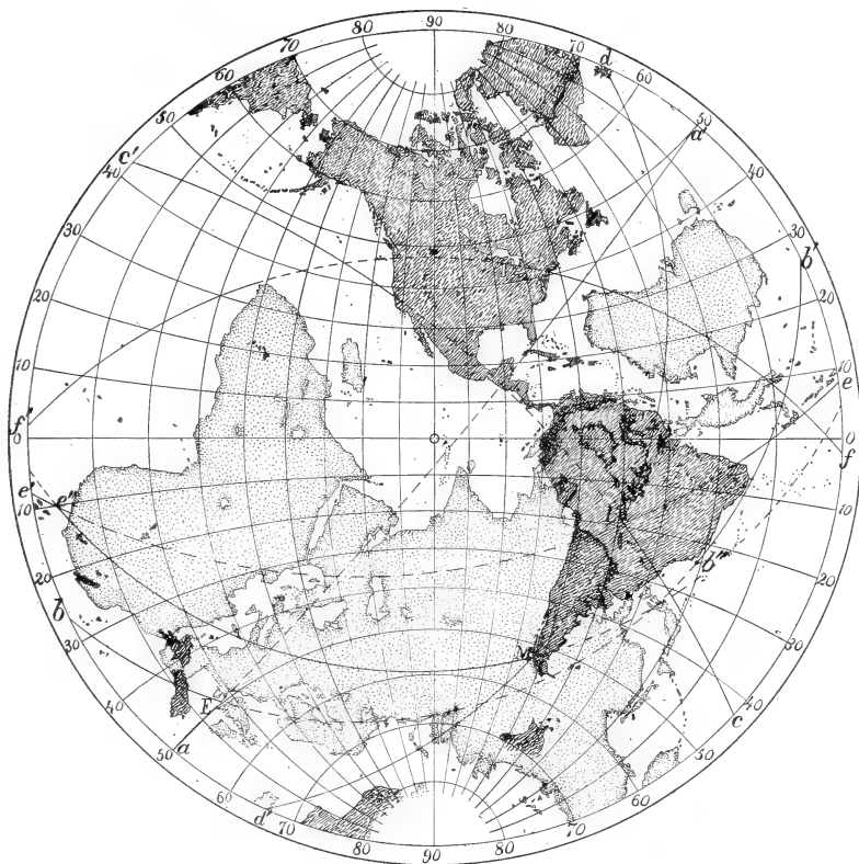
Stereographic Map of the World. Any point on one hemisphere covers the antipodal point on the other.
