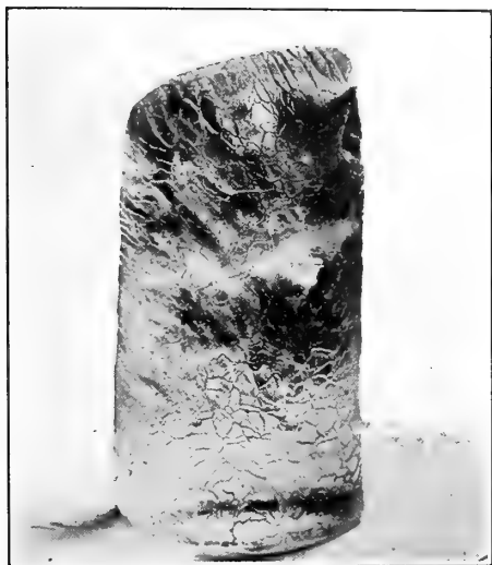
FIG. 3. Same ice cylinder as shown in fig. 2 after reduction in size by slow melting and evaporation (mostly latter) in outdoor laboratory. Note outlines of crystals as shown by etching out of crystal boundaries into distinct grooves. Natural size approximately 8 in. high by 4 in. wide, original cylinder 12 in. by 5 in.
