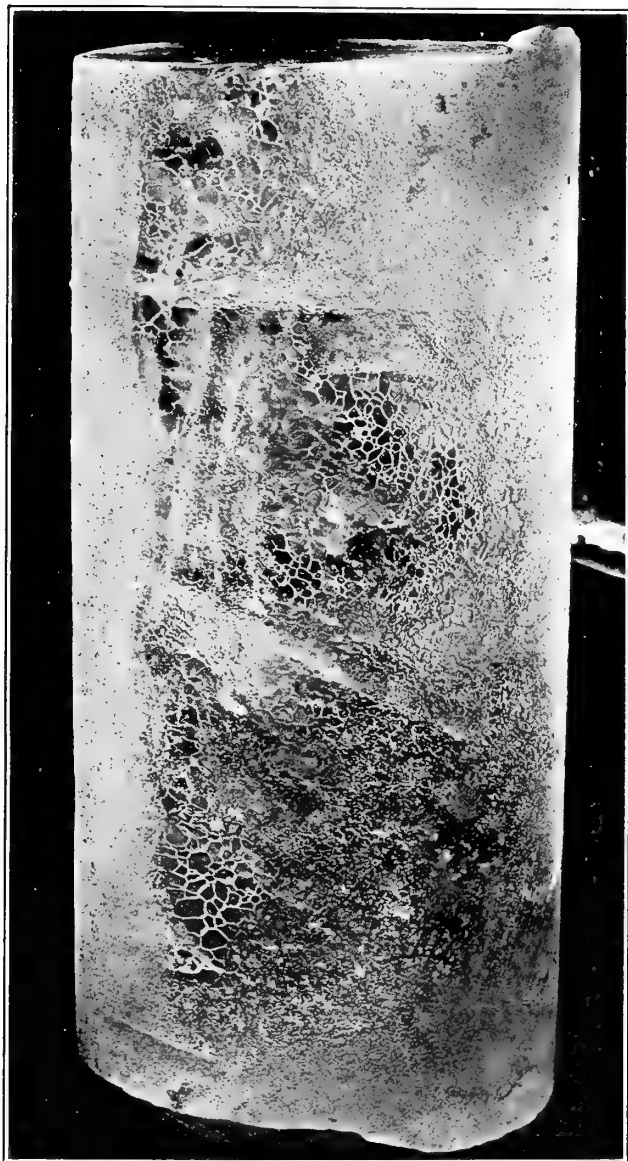
FIG. 2. Ice compressed for 94 hours at air temperatures ranging between -4^{\circ}\text{F.} and 20^{\circ}\text{F.} , under pressures up to 1400 lbs. per square inch. Photographed immediately after removal from copper cylinder. Note that there is no distortion from the cylindrical shape. Note also the etched outlines of the outcropping ends of the crystals.
