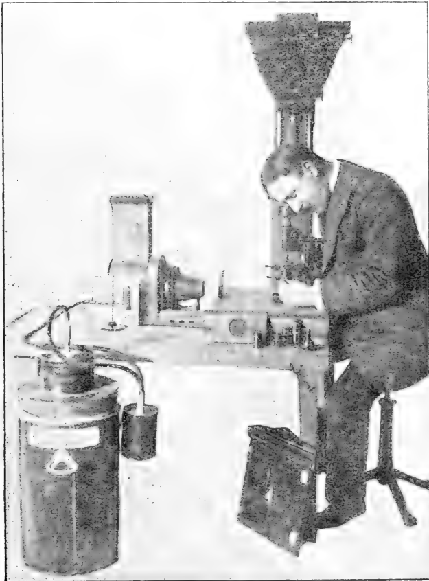
Fig. 2.—Apparatus arranged for photomicrography with acetylene light. To show the acetylene burner it is placed outside the lantern. The camera is racked up so that the operator may arrange the object and substage.
