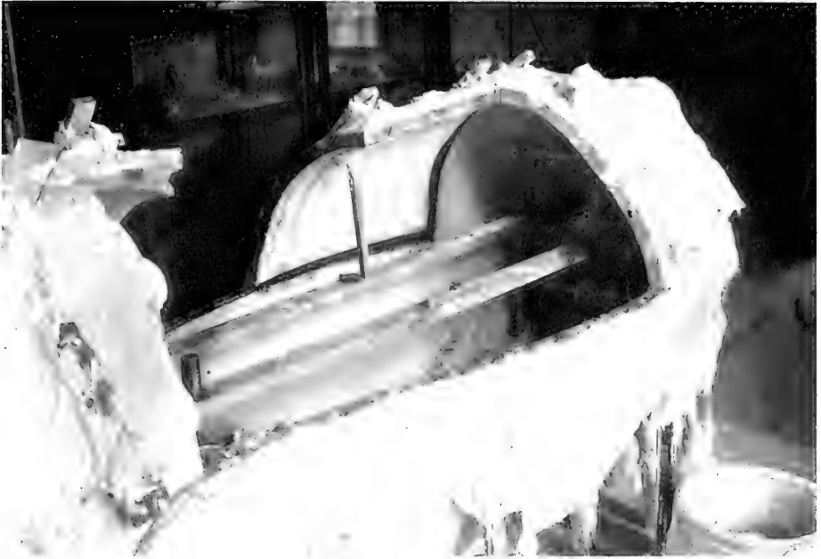
A portion of the piece mold with clay model removed. This has on its interior, of course, a perfect impression of the hippo model, and will give a positive or cast of this impression to soft plaster placed against the interior. The mold of the hippo was thirteen feet long
