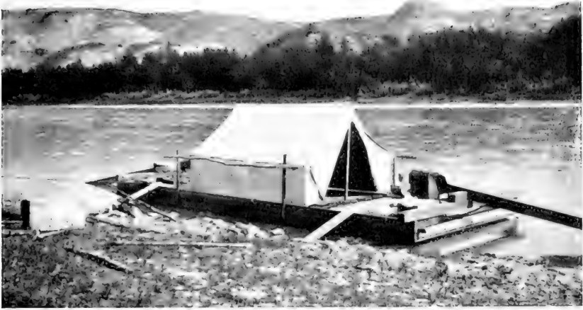
Flatboat constructed for drifting down Red Deer River. A twenty-two-foot sweep at each end, like a long oar, served in guiding the boat out of the way of rocks in the course. This was eventually converted into a houseboat because of excessive rains and dearth of camping places along the shores
