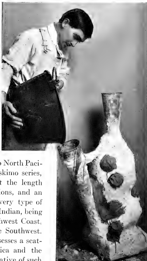
Mr. James C. Bell, expert worker in plaster, making a glue mold of an Indian head. Glue is poured into the funnel, the lower end of which opens into a half-inch space between the original model and the plaster jacket fitting over it. As the glue rises in this space about the model, holes previously cut in the jacket to allow the escape of air are plugged with clay. Finally the funnels at the top and side are capped with clay and the glue is allowed to set for twelve hours
