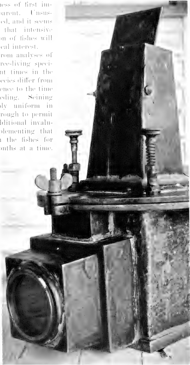
Camera container for submarine photography. The mirror projecting in rear view from the top of the focusing hood enables one without bending over to see the doubly reflected image of objects within the field of the camera. The rods with milled heads are for focusing and for releasing the shutter. Both are protected by stuffing boxes. A soft rubber gasket lies between the cover and the body of the box. All other points are permanently sealed by solder or cement. The cubical body of the box is eight inches on the side, and the weight of the whole apparatus in air is about fifty pounds.
