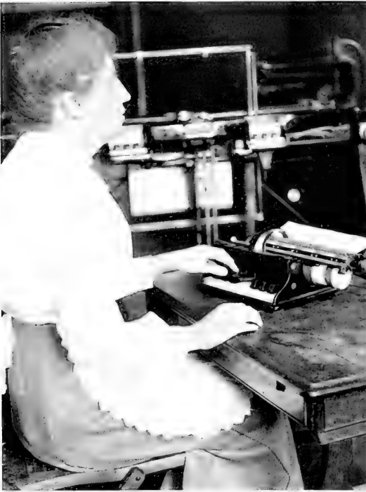
A blind girl is operating the Braille typewriter which uses a system for the blind invented by a French teacher, Louis Braille, in which the characters are represented by raised dots. The "touch method" in typing here reaches the point of perfection
