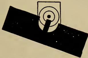
RIFLE LEANED OR CANTED TO RIGHT. BULLET STRIKES LOW, AND A LITTLE RIGHT.
