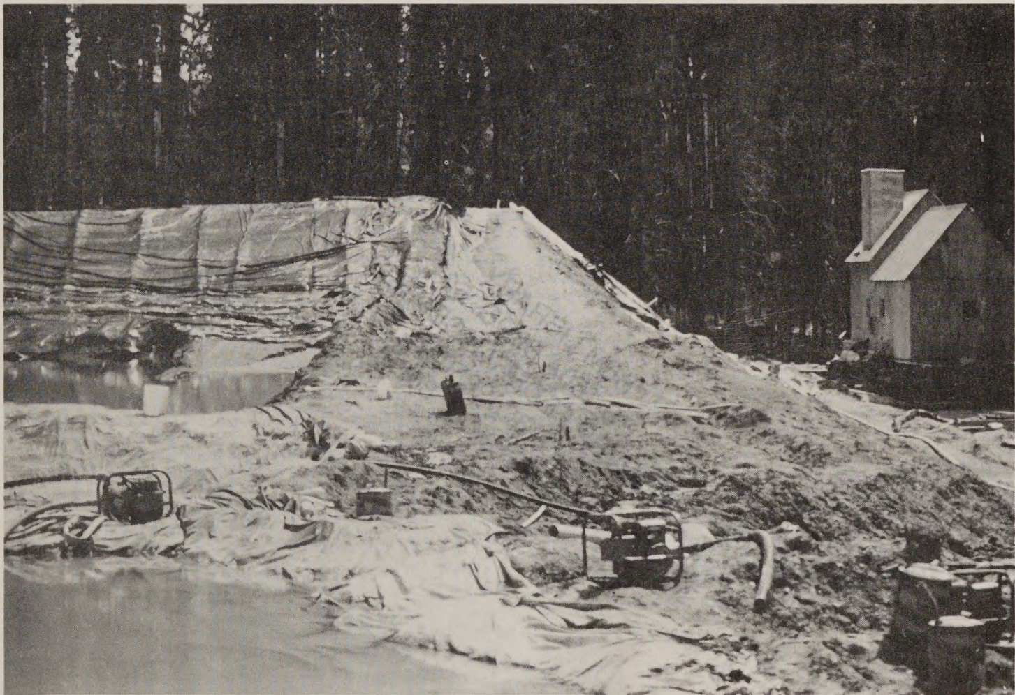
11. Gold heap-leaching processing adjacent to an anadromous fish stream is subject to cyanide leakage.
