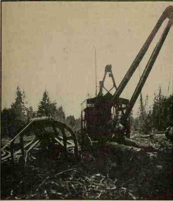
FIG. 4A—12x12 MCGIFFERT LOADER (JAMMER) AND 10-TON TRACTOR DRAWING FAIRLEAD ARCH
