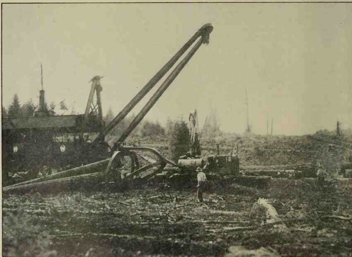
FIG. 6—MCGIFFERT LOADER ("JAMMER") AND TRACTOR ARCH UNIT AT LANDING
