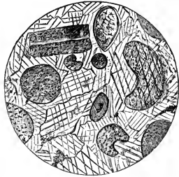
Fig. 12.—Section of Coniston Limestone (Lower Silurian) from Keisley, Westmoreland; magnified. The matrix is very coarsely crystalline, and the included organic remains are chiefly stems of Crinoids. (Original.)
