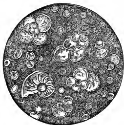
Fig. 7.—Section of Gravesend Chalk, examined by transmitted light and highly magnified. Besides the entire shells of Globigerina , Rotalia , and Textularia , numerous detached chambers of Globigerina are seen. (Original.)
