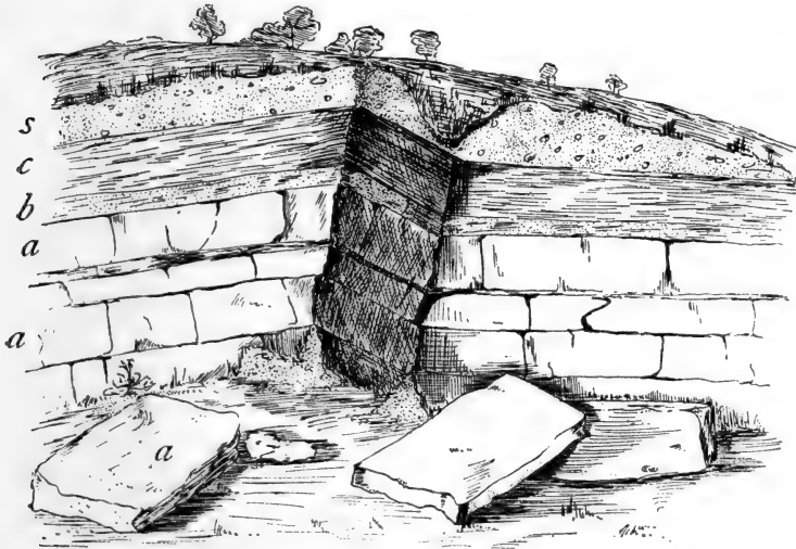
Fig. 1.—The Face of a Quarry, showing layers or "beds" of different rock, a , b , and c . The top gravel and soil s has been disintegrated by the growing plants and atmosphere.
