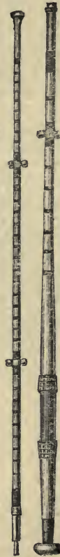
Fig. 19. The Author's Light Sea Rod with a double set of Porcelain Rings. Exaggerated to show details. Length 7ft.; diameter of middle of butt, \frac{3}{16} in.; of top, \frac{1}{4} in.
