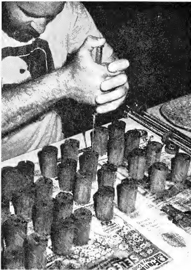
Filling feeder segments with gum arabic solution using a syringe with a long needle to ensure filling the entire cavity from the bottom up. (Photo: Lee Miller)
