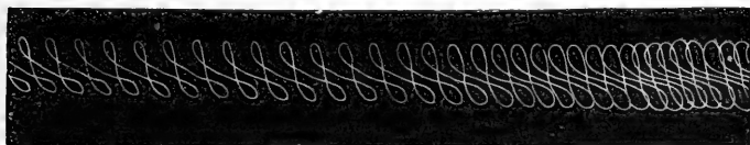
FIG. 76.—Tracing of a Wheatstone's kaleidophone rod, tuned to the octave, that is to say, vibrating twice transversely for each longitudinal vibration. (This figure is taken from R. Koenig.) The slackening speed of the cylinder produces an approximation of the curves towards the end of the figure.
