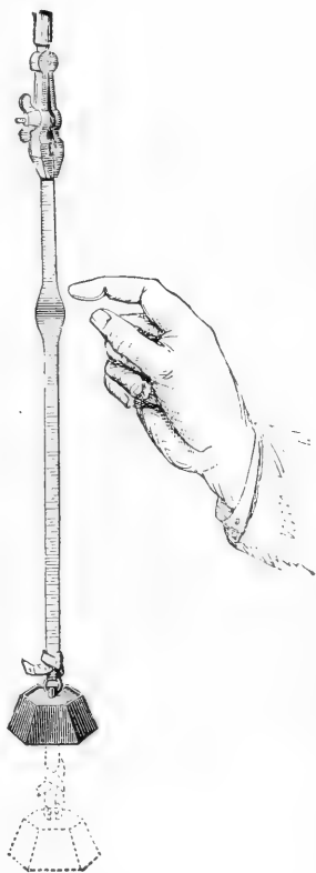
FIG. 9.—Transformation of heat into work by a strip of india-rubber.
