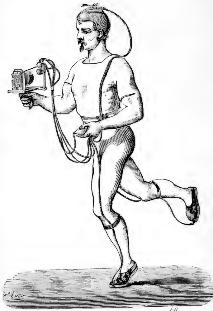
FIG. 27.—Runner provided with the apparatus intended to register his different paces.
