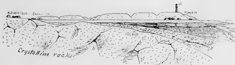
FIG. 7. Ideal section from Maceio to Albuquerque, 35 kilometers, along the Alagôas Railway, showing the coast sediments resting on the crystalline rocks.
