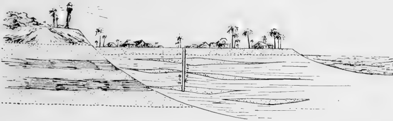
FIG. 14. Section showing the relation of the deep well at Maceio to the rocks of the hills above the city.
