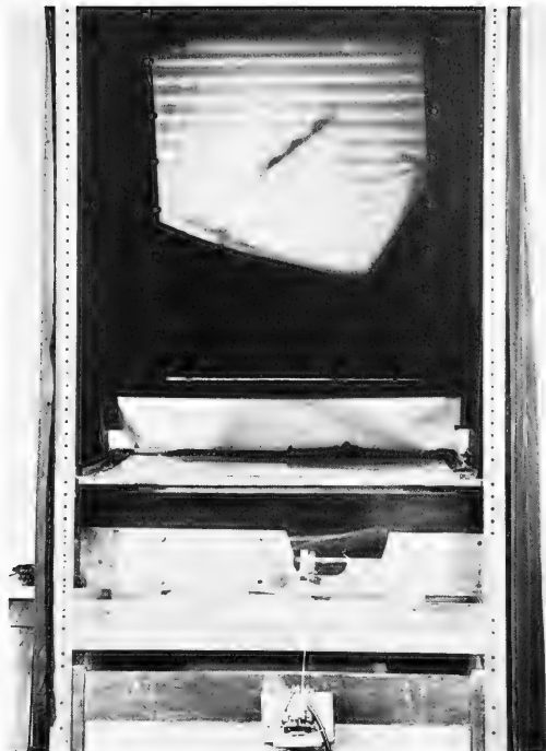
FIGURE 2. RIPPLE TANK-SCREEN SHOWING EXAMPLE OF WAVE REFRACTION, DIFFRACTION AND REFLECTION
