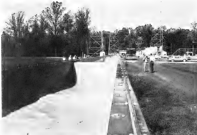
FIGURE 12. A SIX-FOOT WAVE IN 635- FOOT TANK
