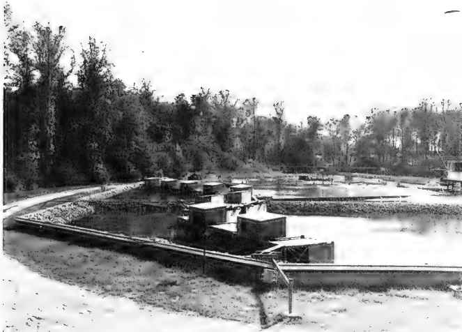
FIGURE 8. SHORE PROCESSES TEST BASIN, CONTAINING NINE SEPARATE WAVE GENERATORS
