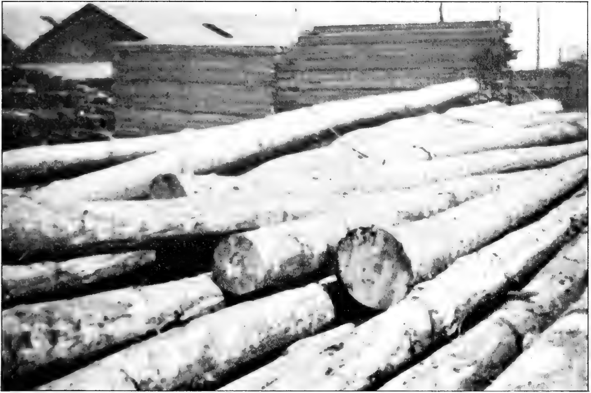
LONG PILES AWAITING TREATMENT.
