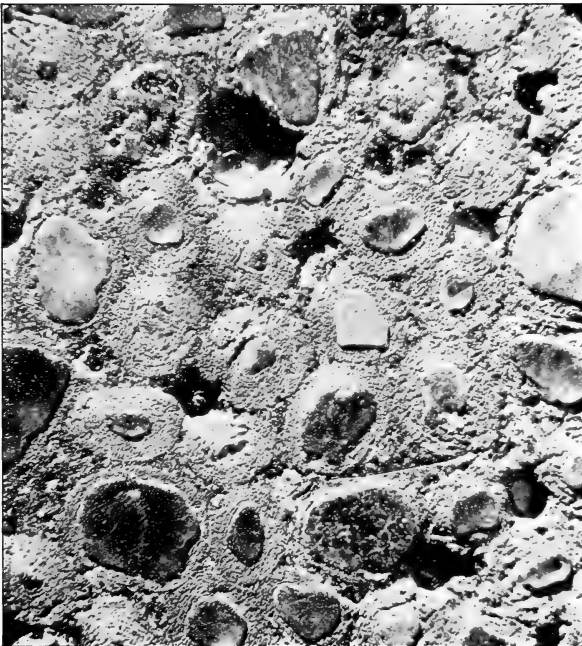
Oolitic ore, magnified so as to show quartz nuclei and concentric structure
