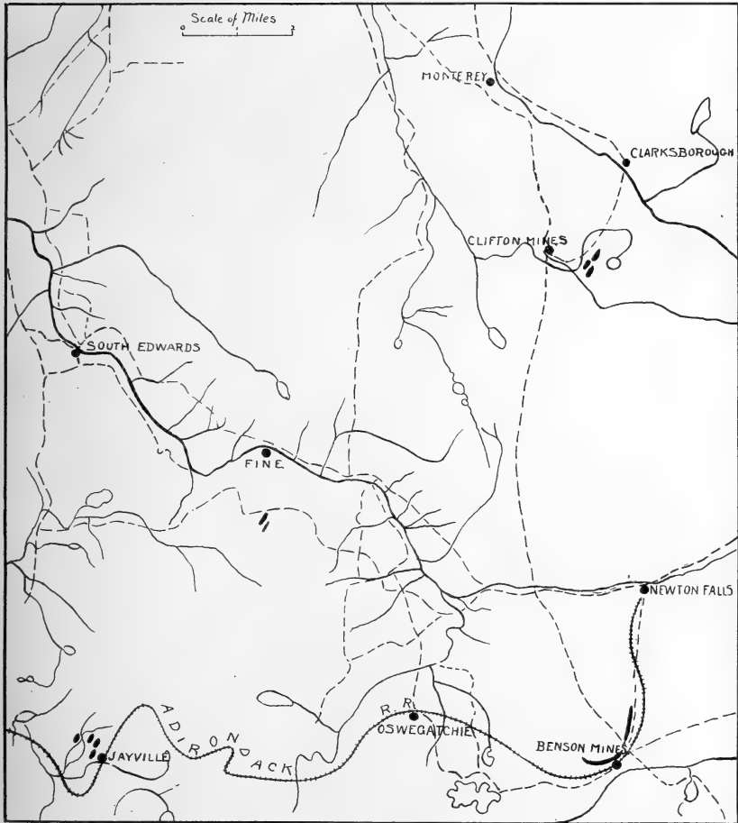
Fig. 21 Sketch map of the St Lawrence county magnetite deposits. Ore bodies shown by heavy lines
