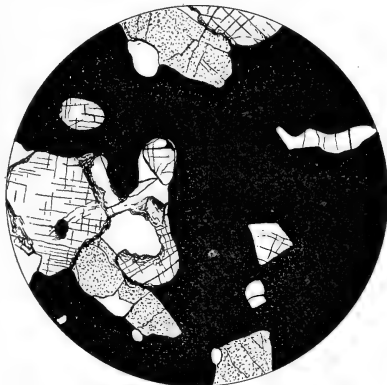
Fig. 28 Old Bed ore. The black is magnetite; the stippled mineral is apatite; the lined mineral is emerald-green pyroxene. Actual field 0.1 inch.
