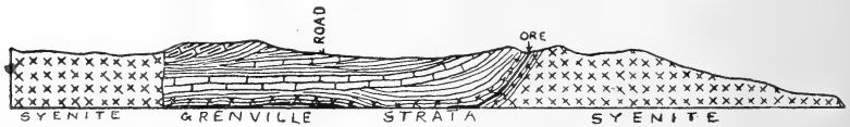
Fig. 18 Cross section at the Cheever mine, in a direction n. 60^{\circ} e.
