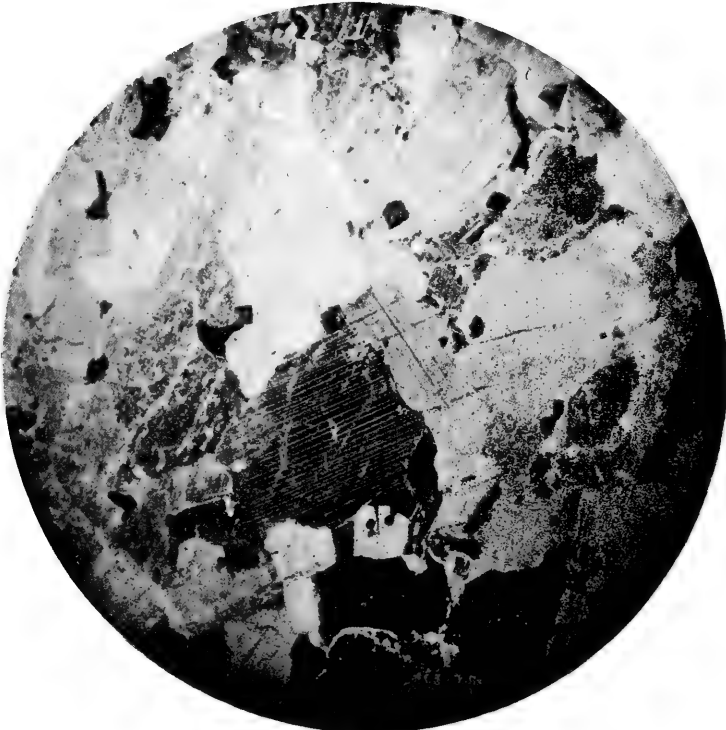
Photomicrograph of anorthosite, Split Rock. The main component is labradorite which appears striated. Enlarged 22 times.
