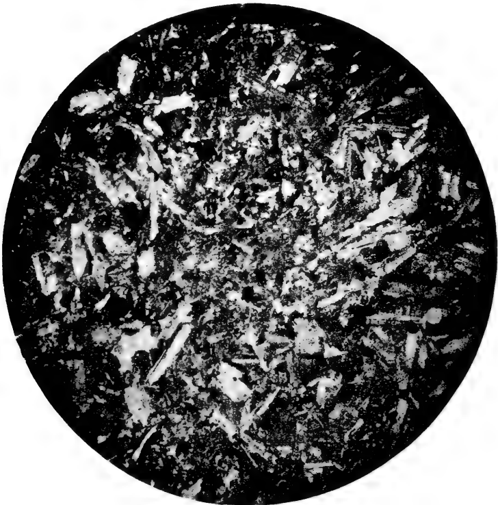
Photomicrograph of diabase, Fort Ann. Lath-shaped crystals of feldspar in a groundmass of pyroxene. Enlarged 22 times.
