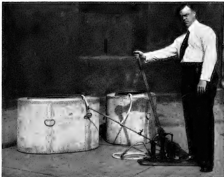
HAND AIR COMPRESSOR FOR THE AERATION OF SHIPPING TANKS
