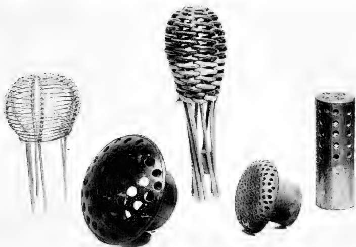
FIVE TYPES OF STRAINERS USED IN THE AQUARIUM TO PREVENT ESCAPE OF SPECIMENS FROM TANKS
