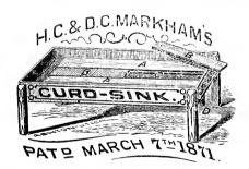
This Sink has a bottom (A) sloping from each side to the center which is arranged with a snaken channel (C) running its entire length. Said channel is covered with a movable metalic strainer (B). A spont (D) conducts away the whey as it drains off from the curds in the sink.
