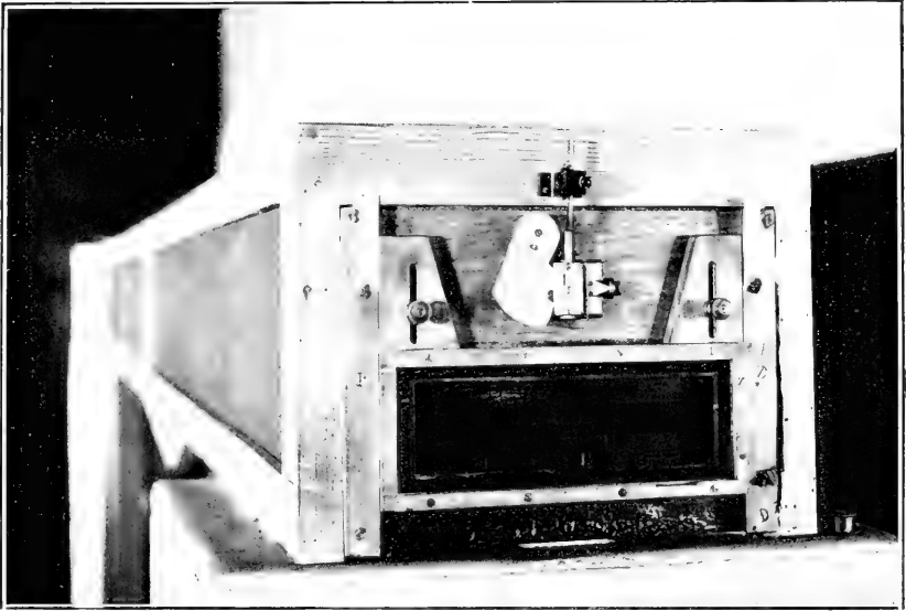
SLIT AND PLATE-HOLDER END OF SIMPLE WOODEN SPECTROGRAPH OF LITTROW OR AUTO-COLLIMATING TYPE (18 FEET FOCAL LENGTH), USED IN THE SPECTROSCOPIC LABORATORY ON MOUNT WILSON.
