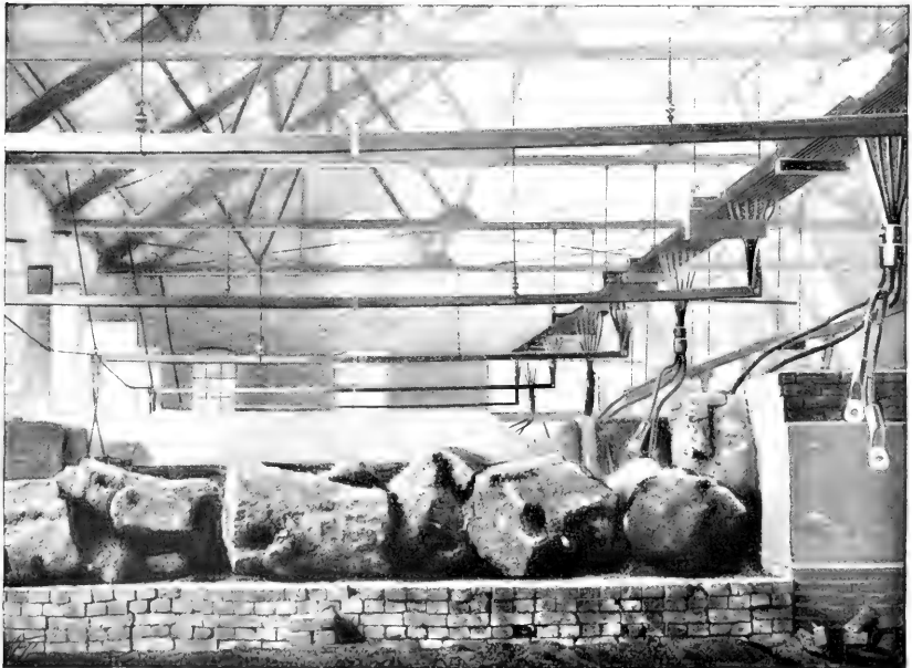
A CARBORUNDUM FURNACE AFTER A RUN.
