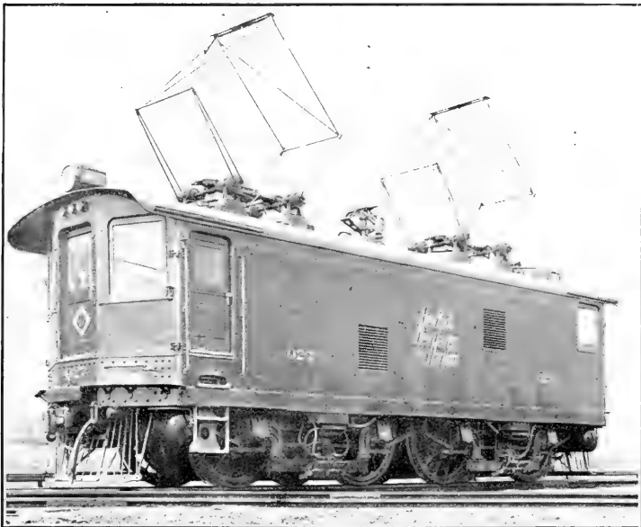
NEW HAVEN 1,000-HORSEPOWER ALTERNATING-CURRENT ELECTRIC LOCOMOTIVE.
