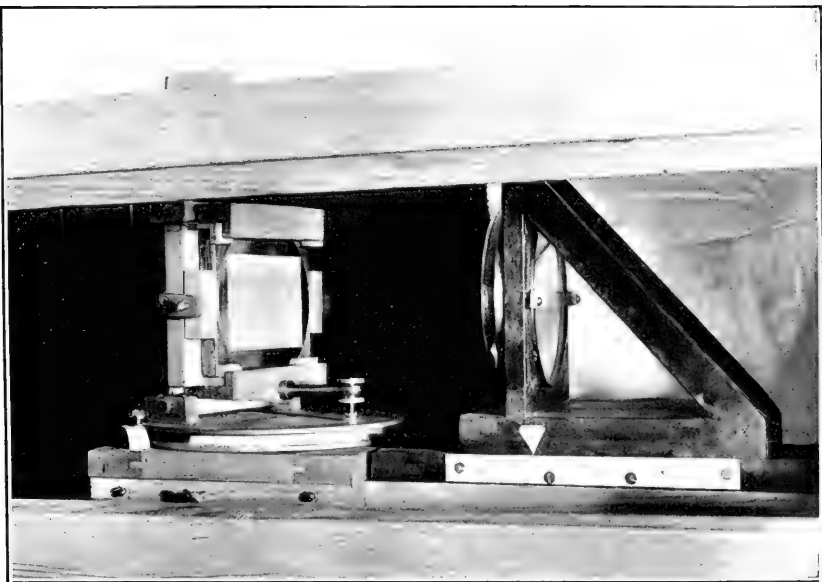
GRATING AND LENS SUPPORTS FOR MODERN SPECTROGRAPH (18 FEET FOCAL LENGTH), USED IN THE SPECTROSCOPIC LABORATORY ON MOUNT WILSON.
