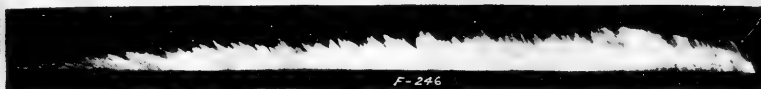
R.P.M. 375. DURATION OF FLAME 1539. MILLISEC. HEIGHT OF FLAME 50.21 IN. A BLACK BLASTING POWDER.
