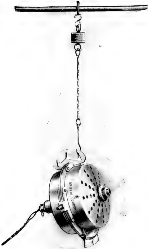
FIG. 8.—MOTOR-GYROSTAT PRECESSING ON CHAIN SUPPORT.
