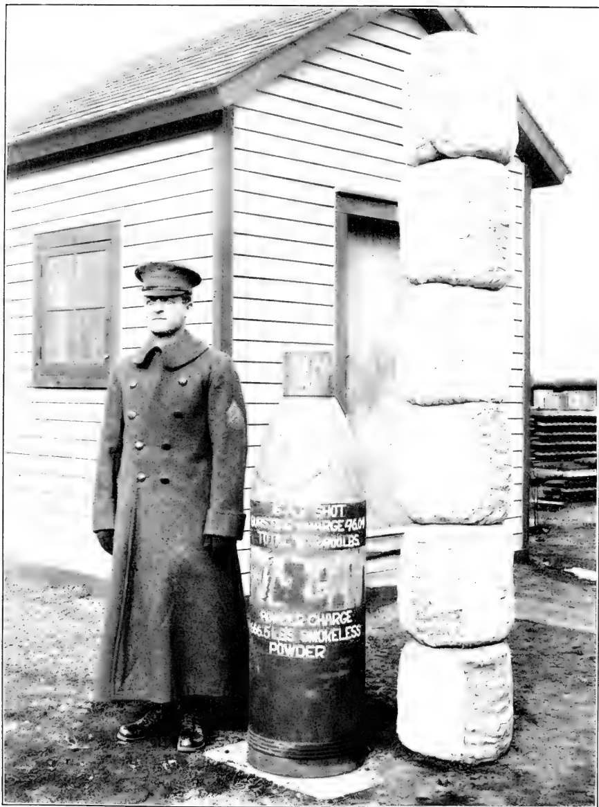
PROJECTILE AND POWDER CHARGE FOR 16-INCH GUN. WEIGHT OF PROJECTILE, 2,400 POUNDS; WEIGHT OF POWDER CHARGE, 666.5 POUNDS OF SMOKELESS POWDER.
