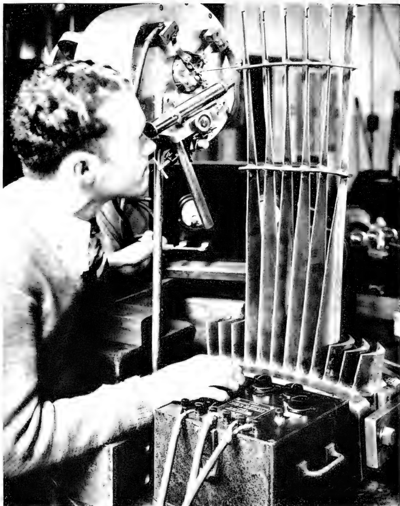
RESEARCH STUDIES OF VIBRATION IN LARGE STEAM TURBINE BLADES.
