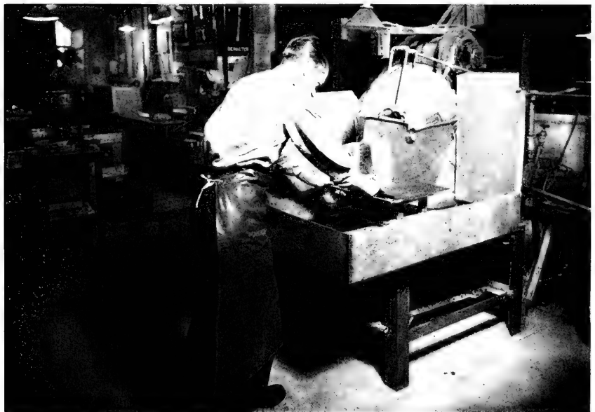
2. CUTTING OPTICAL GLASS BY MEANS OF A 24-INCH DIAMOND SAW
