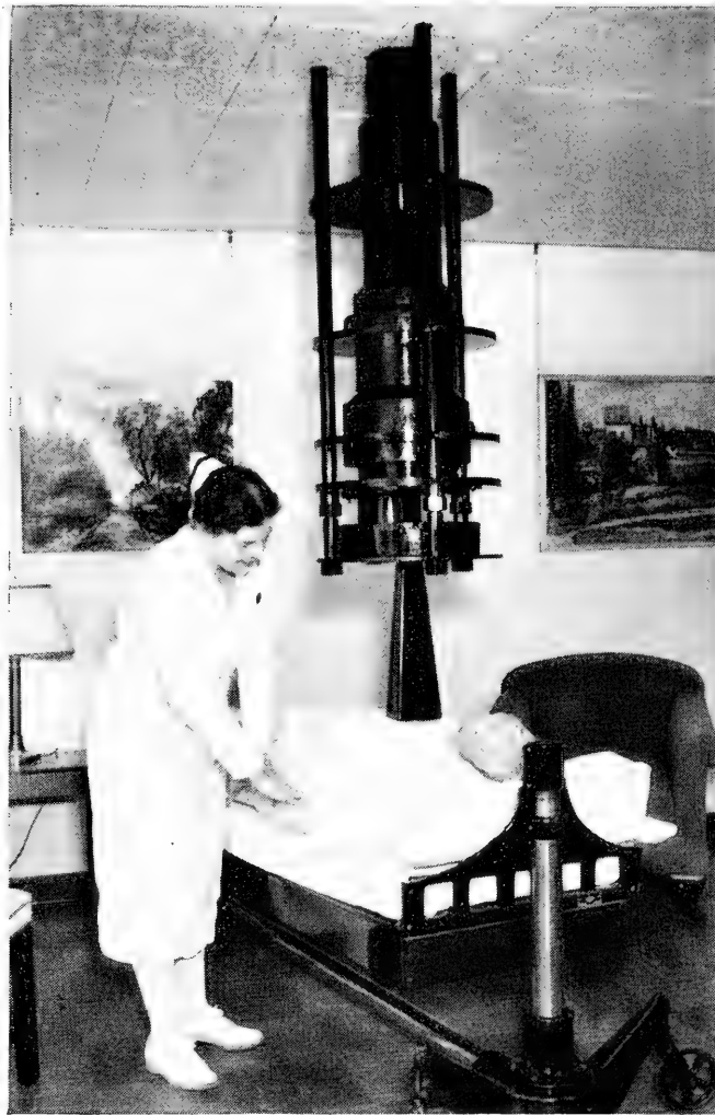
Pioneering work in radiation with X-rays produced by over 1 million volts was made possible by the M. I. T.-designed air-insulated electrostatic generator at the Huntington Memorial Hospital. More than 1,000 patients have been treated with this unusual equipment which established many of the advantages of supervoltage radiation for deep cancer therapy.
