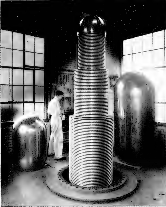
The column and terminal structure of the 3-million-volt generator at M. I. T. with its tank removed. This generator produces voltages over 10 times higher than the standard voltage for deep X-ray therapy. Its radiation output, more penetrating than gamma rays of radium, is equivalent to several times the total world supply of that precious material.
