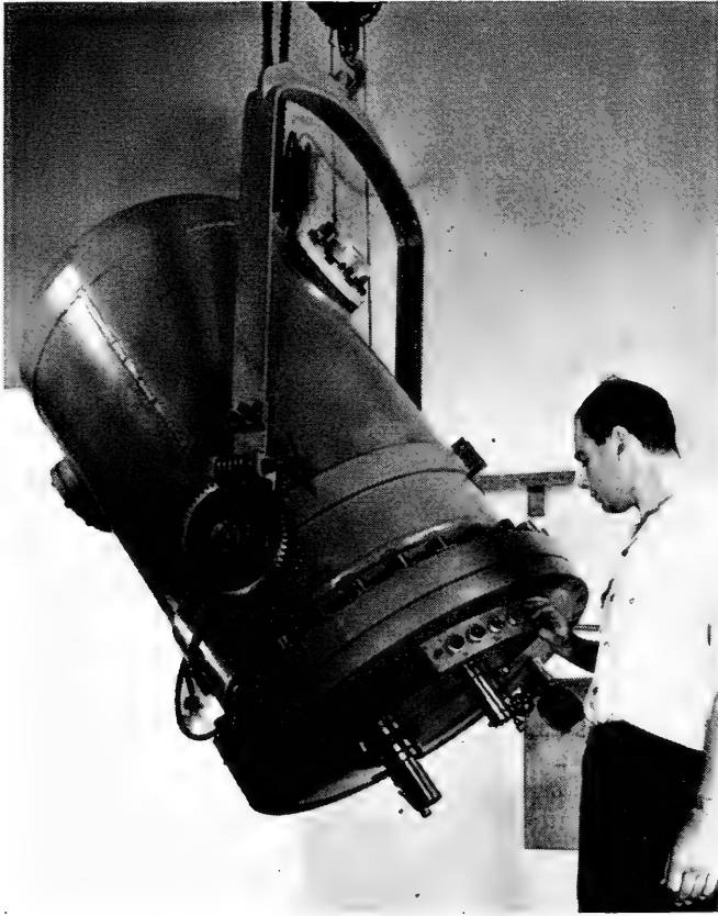
This supervoltage X-ray generator, the most compact machine thus far developed for cancer therapy, is comparable in size and flexibility of use to lower-voltage equipment now generally available. It was developed at M. I. T. under a grant by the American Oncologic Hospital which will use it in its program of deep therapy.
