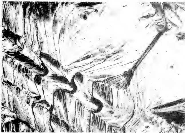
FIG. 2. Fracture surface of metal, showing the external surface of a grain (grain boundaries). Oxide was deposited on growths which strongly affect the forgeability. The growths are in the form of thin plates which are carbides, the essential factor for forgeability. The oxide was removed by the vacuum treatment. The oxide was removed by the vacuum treatment. The oxide was removed by the vacuum treatment. Magnified 385 times.
