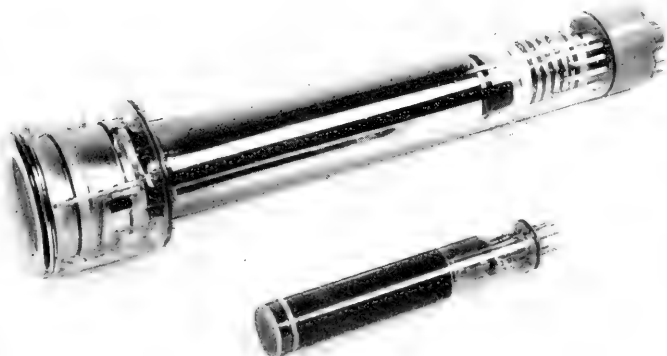
2. SIZE REDUCTION AND SIMPLIFICATION IN TELEVISION PICK-UP TUBES: THE IMAGE ORTHICON AND THE VIDICON
