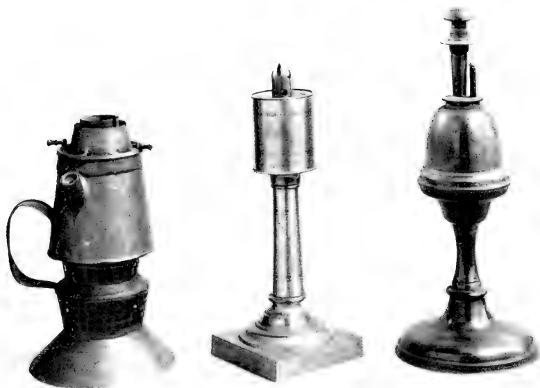
Patent models illustrating inventive ingenuity: Left , Rosin lamp, with heater underneath to keep the rosin fluid, patented by Prentice Sargent, Newburyport, Mass., March 4, 1856. Middle , Lard lamp patented by Silas B. Terry, Plymouth, Conn., February 24, 1843. Right , Fluid vapor lamp patented by C. A. Green, Philadelphia, April 21, 1857. The small burner seen at right superheated the volatile fuel in the large burner, causing it to vaporize and burn as a gas.
