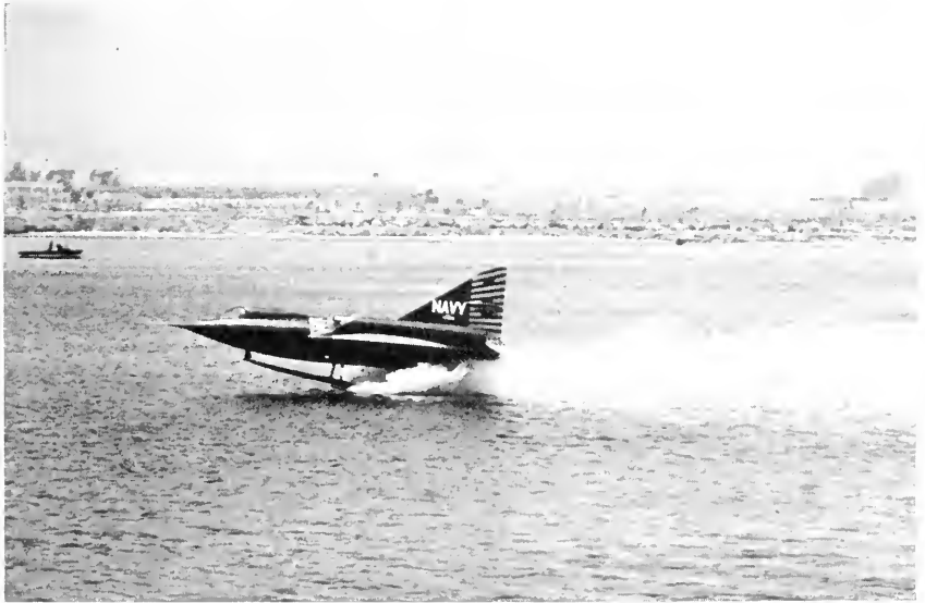
2. Convair Sea Dart. Jet engines and skis accomplish this change from an awkward float seaplane to a sleek supersonic design that suffers no disadvantage from being water-based, and has many advantages.
