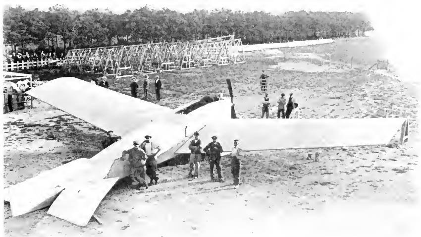
2. Forty years ago this highly streamlined cantilever-wing Antoinette was a forerunner of present-day construction, but at the time, the design was ignored.
