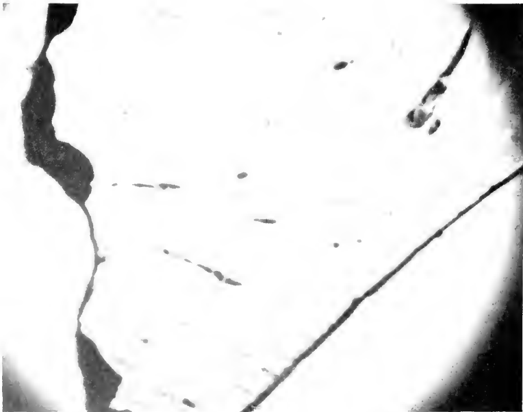
1. Georgia tektite, illustrating the inhomogeneity of a thin polished section by means of transmitted light
