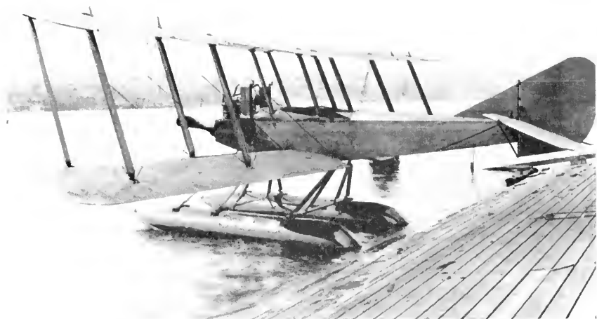
1. An early Boeing training plane. Note low rudder, small fin, short tail length, no stabilizer. This was typical of the 1910-1914 era.
