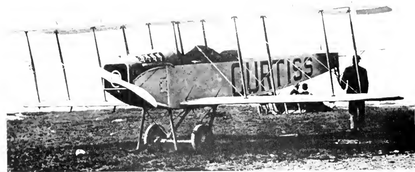
2. This 1913 Curtiss tractor had a typical landing gear of skids and wheels. On a hard landing, the skids would break and turn the plane over.
