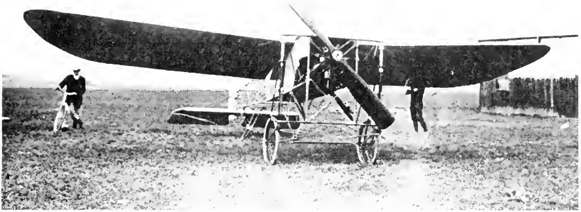
1. The 1909 Bleriot monoplane. Tractor engine location, warping wings for lateral control, rear elevators and tail.
