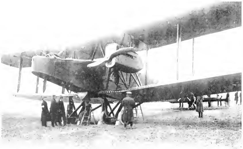
2. The Handley-Page of World War I. This widely used twin-engine plane typifies the configuration of engine between the wings at this early stage.
