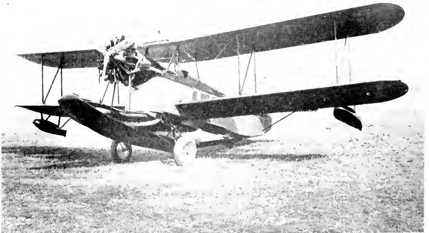
2. The practical retractable gear of the amphibian in 1923-1933 led to a much wider adoption of this feature on land planes.
