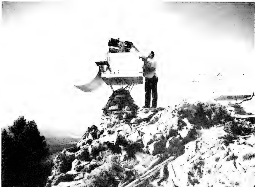
1. Scanning photometer on Fritz Peak, Colo., for measuring the intensity of airglow and its changes. (Photograph courtesy National Bureau of Standards Boulder Laboratories.)
