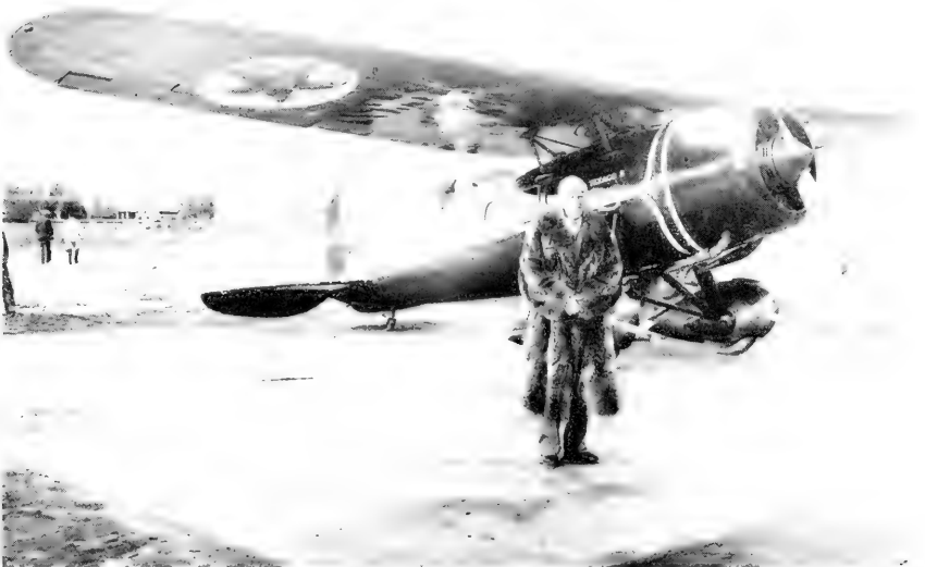
2. Cowed radial engine on Lockheed Air Express , with Frank Hawks, 1929.
