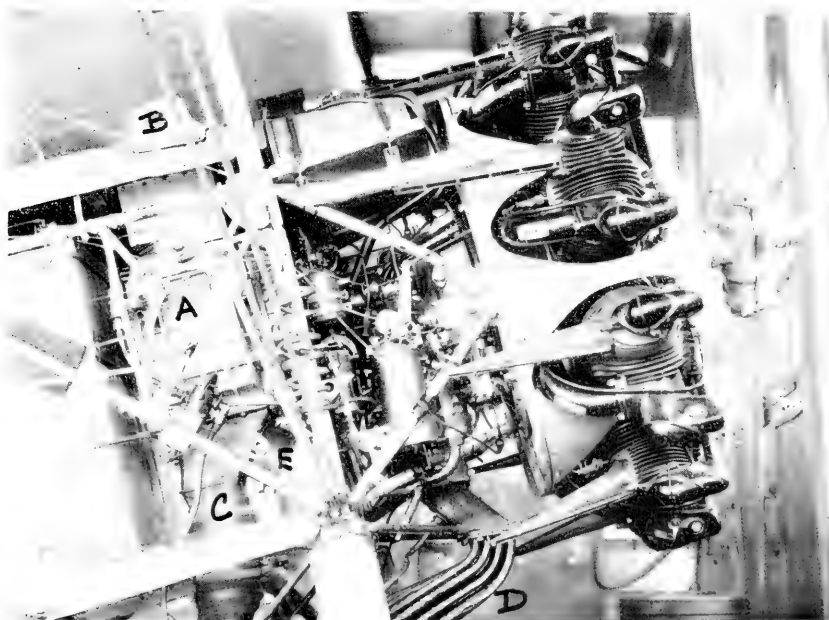
2. N.A.C.A. Roots type supercharger, coupled to Pratt & Whitney "Wasp" engine in a Wright Aero. Corp. "Apache" airplane. This installation broke the world altitude record in 1927. This was the only successful displacement-type supercharger. A, Supercharger; B, air intake; C, delivery pipe through intercooler D; E, supercharger bypass.
