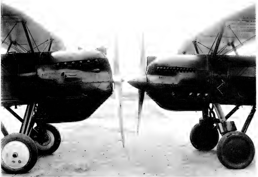
1. Comparison of radiator installations for water (left) and Ethylene Glycol cooling, on Curtiss Falcon airplanes, 1930. (Courtesy Curtiss-Wright Corp.)
