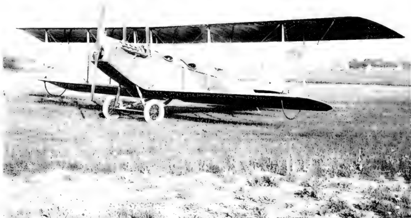
2. Curtiss JN-4 airplane with OX-5 engine.
