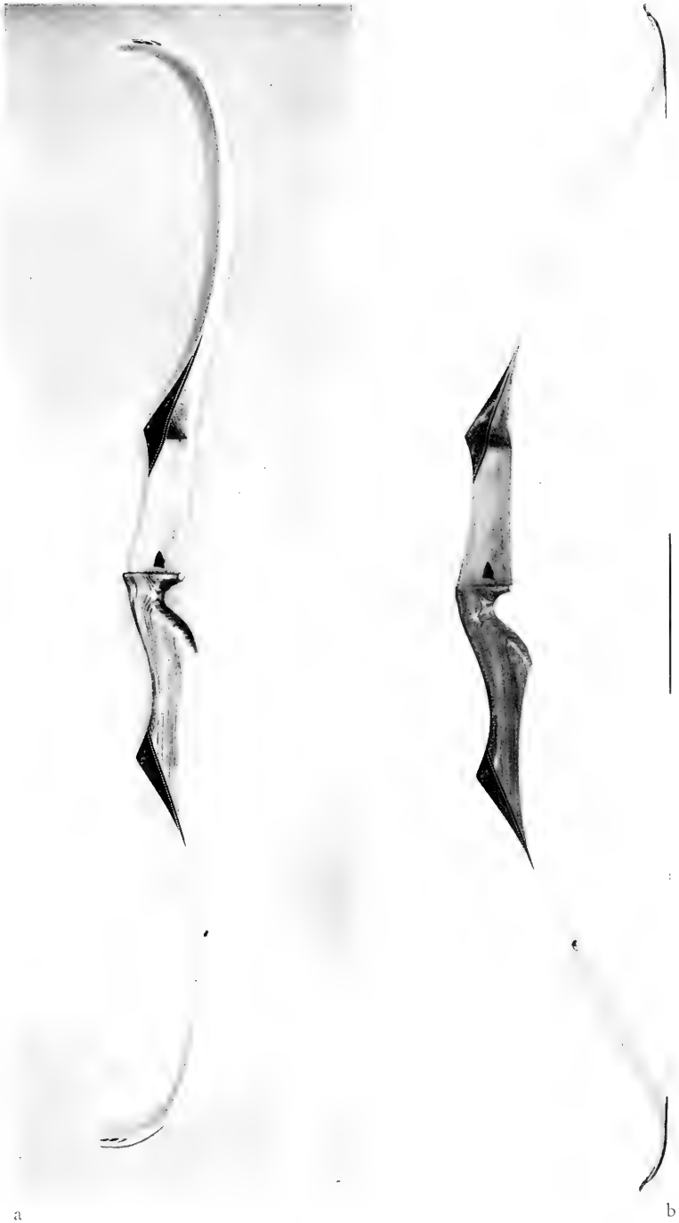
A modern composite bow (bow of the 1960's) (a) relaxed, (b) braced, and pl. 5, at full draw. Note the length (ca. 20") of the equal limbs, as compared with the 34" length of the upper and 32" lower limb of the English longbow of figure 1, and the rigid midsection, 27" long, which is completely absent in the English longbow. (Photos courtesy of Bear Archery Co.)
