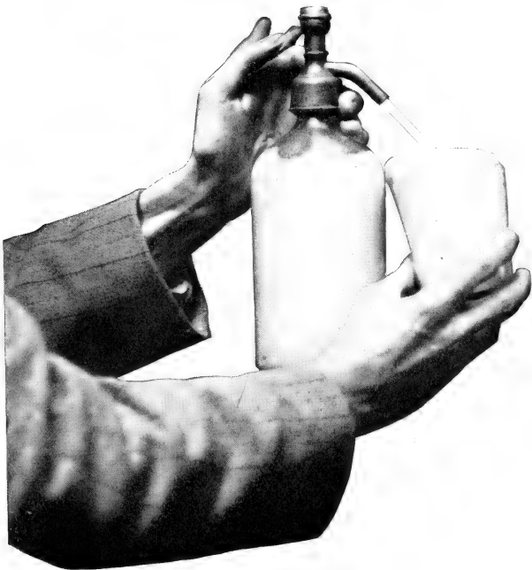
FIG. 6. APPARATUS USED FOR CARBONATING MILK. PRESSURE 150 TO 175 LBS. TO SQUARE INCH.
