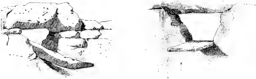
FIG. 39. Single stone roof drains.
