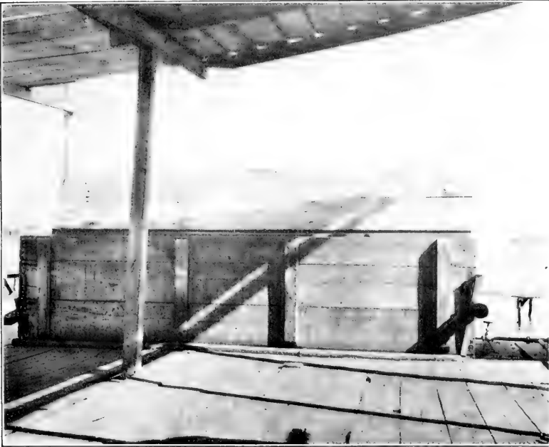
FIG. 1.—ONE FORM OF BOX OR WOODEN COOKER, USED AT POINTS IN MARYLAND.
