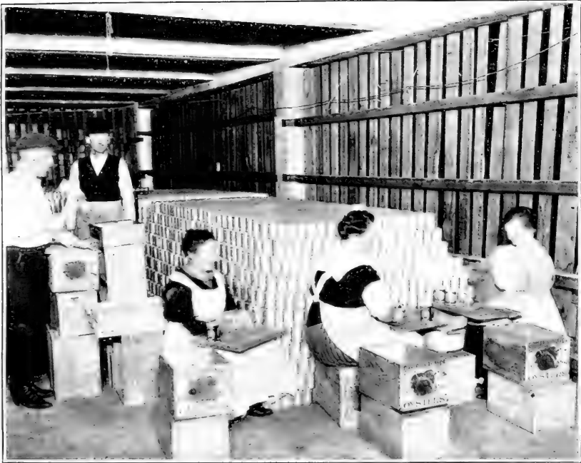
FIG. 1.—INTERIOR OF OYSTER CANNERY; LABELING AND BOXING CANS OF OYSTERS.
