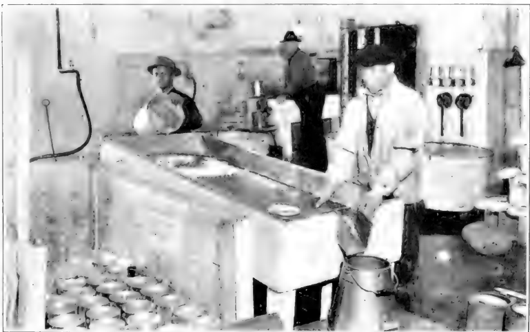
FIG. 2.—WASHING FRESH OYSTER MEATS ON "SKIMMING BOARD."
