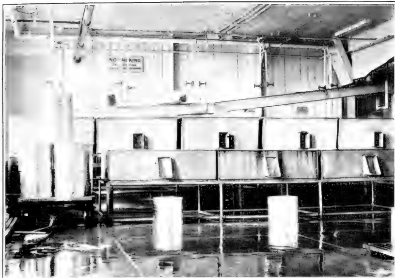
FIG. 1.—TANKS FOR WASHING SHUCKED OYSTERS.
