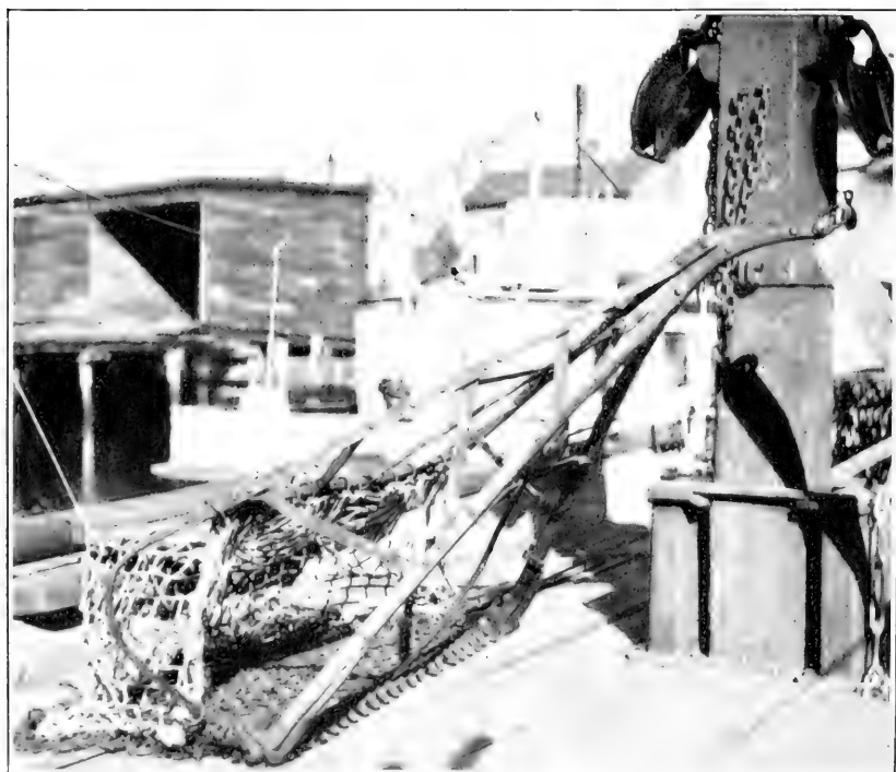
FIG. 2.—MACHINE-HOISTED DREDGE USED IN TAKING OYSTERS.
