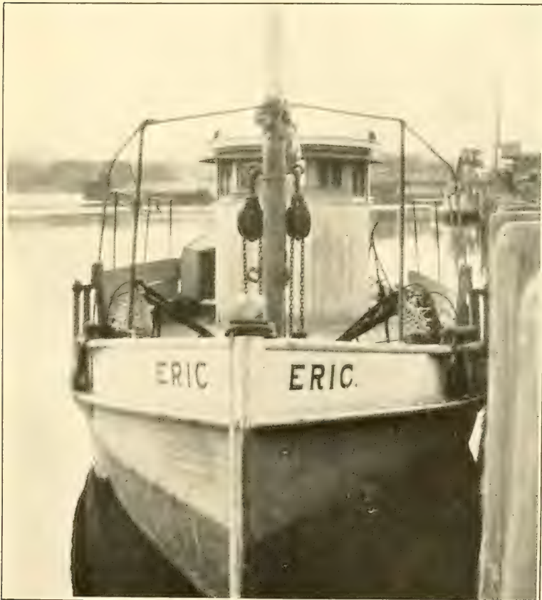
FIG. 2.—GASOLINE BOAT USED IN DREDGING OYSTERS IN LONG ISLAND SOUND.
