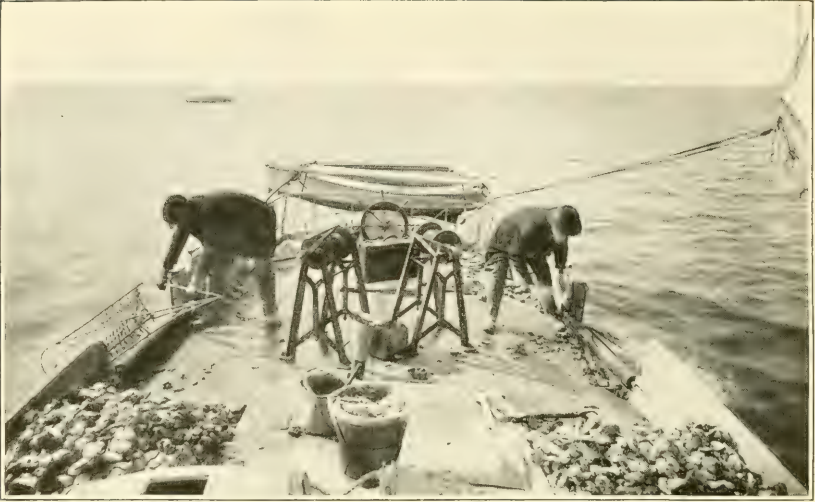
FIG. 1.—HAND DREDGES AND WINCHES FOR HOISTING THEM. (Photo from Prof. E. N. Cory, Maryland State University.)
