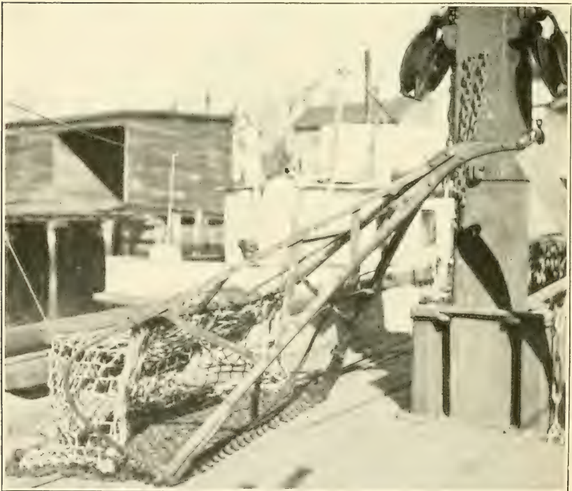
FIG. 2.—MACHINE-HOISTED DREDGE USED IN TAKING OYSTERS.
