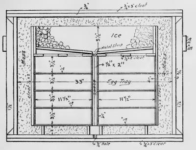
FIG. 8.-Atkins-Dinsmore shipping case. Longitudinal section.
