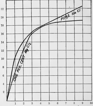
FIG. 2.—Curves show retardation of penetration of salt due to 1 per cent of magnesium chloride impurity (section ½ to 1 cm. depth). Figures at left indicate per cent of chlorine in dry fish; at bottom, time in days.
