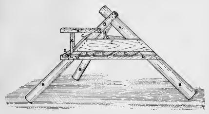
FIG. 1.—Three-legged rack horse or trestle: A., horse head; B.B., horse legs; C.C.C., 12-inch boards to make sides of crib and also to act as braces; D.D.D., leg braces which also support bottom of crib; E.E.E., bottom of crib; X.X., bracket for supporting walk.
