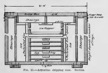
cork. Two cleats seven-eighths by 3 inches are attached lengthwise to the bottom on the outside.
