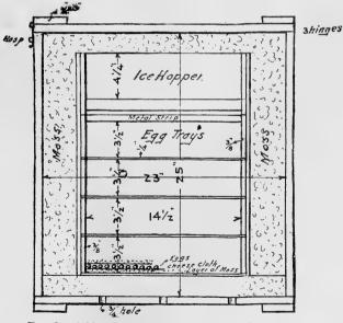
FIG. 9.-Atkins-Dinsmore shipping case. Cross section.
