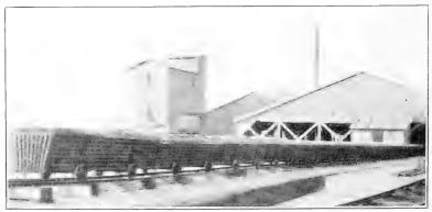
FIG. 3.—FIFTEEN CARS OF OYSTERS READY TO BE RUN INTO THE OYSTER CANNERY. Eac<sup>+</sup> car holds 20 bushels, making 300 bushels in all. The capacity of this cannery is 1,500 bushels per day.
