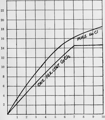
FIG. 1.—Curves show retardation of penetration of salt due to 1 per cent of calcium chloride impurity (section ½ to 1 cm. depth). Figures at left indicate per cent of chlorine in dry fish; at bottom, time in days.
