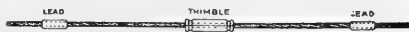
BOTTOM OR LEAD LINE, SOFT MANILA NT 120 LEADS ARE 8" LONG, MADE OF SHEET OF LEAD BEATEN TIGHT ON LINE THIMBLE TURNED IN TWO PIECES TO FIT ROPE AND LASHED ON
