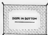
40 MESHES WIDE IN CENTER OF WIDTH; LASHED TOGETHER WITH 1" ROPE; CLOSER TO BOTTOM THAN TO TOP.
