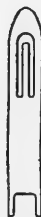
NET MAKER'S NEEDLE; MADE ALL SIZES FROM 3" OR 4" UP TO 2 1/2"; GENERALLY OF HARDWOOD, BUT SOMETIMES OF BRASS OR OTHER MATERIAL
