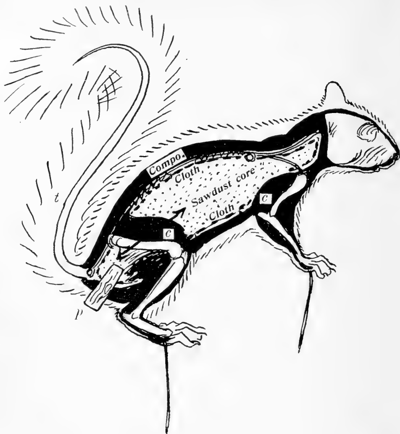
BUILT-IN HOLLOW MANIKIN METHOD FOR MOUNTING SMALL MAMMALS.
