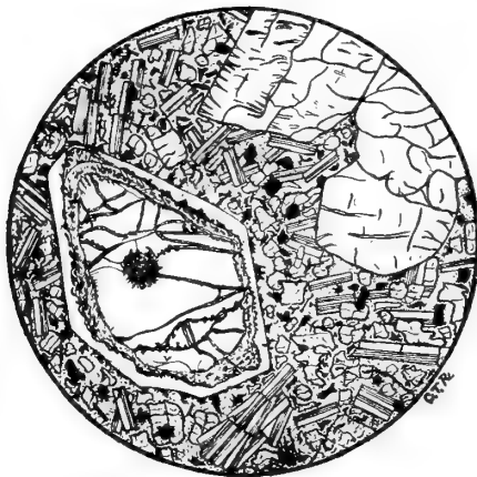
FIGURE 25. Olivine-augite camptonite; showing phenocrysts of olivine in a ground-mass of plagioclase, granular pyroxene and magnetite. (Specimen No. 316.)
