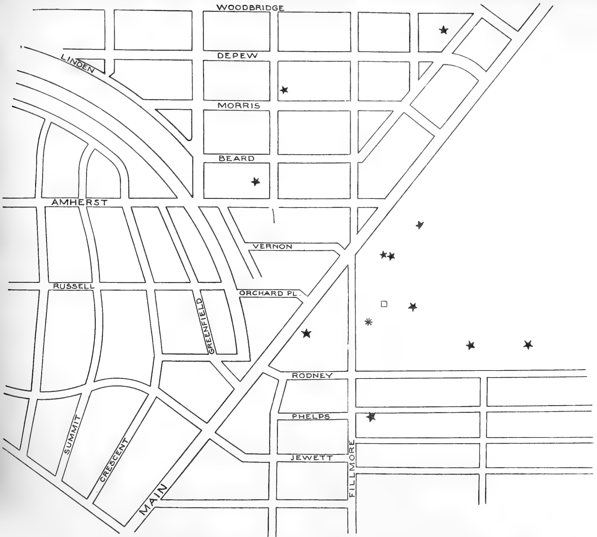
GROUP OF GAS WELLS NEAR THE MAIN STREET CROSSING OF THE NEW YORK CENTRAL BELT LINE, BUFFALO. Productive wells are represented by stars; unproductive wells by double stars.
