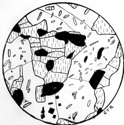
FIGURE 23. Section of hypersthene-gneiss from west side of Sterling lake. The hypersthene is marked with interrupted striations; the magnetite forms irregular black grains and the pyrite square ones. The plain white is plagioclase, containing inclusions of apatite, magnetite and pyrite. (Specimen No. 346.)
