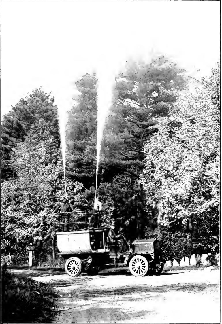
The first power truck sprayer ever invented. Built by the Massachusetts State Forester in 1911 for spraying in the gypsy and brown tail moth work. The whole outfit was designed and built for this work, and promises to revolutionize the question of spraying, particularly road-side, park and shade tree work, in combating insect and fungous depredations. It can be used for forest fire work as well. The same engine that propels the truck also imparts the power for spraying. See description elsewhere.
