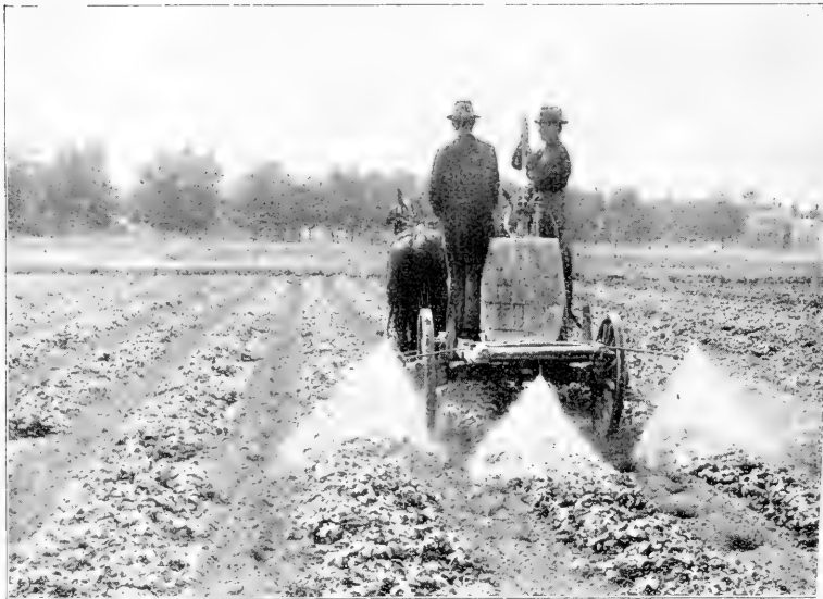
Fig. 101.—Three-row Sprayer at work in field of Strawberries. It is claimed that one man can drive and work the machine. Price of Hose, Piping, Nozzles and Connections (without the pump), $7.50.
