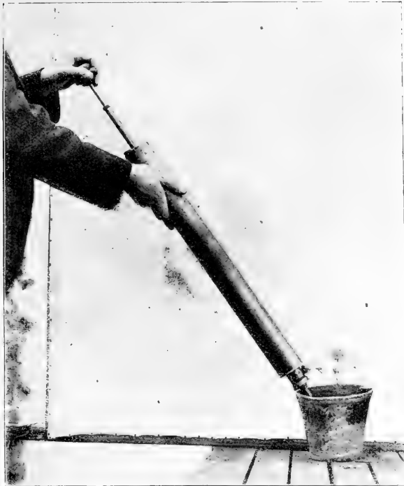
Fig. 117.—McGowen Injector. For putting bi-sulphide of carbon about roots of trees or plants. Slingerland.
