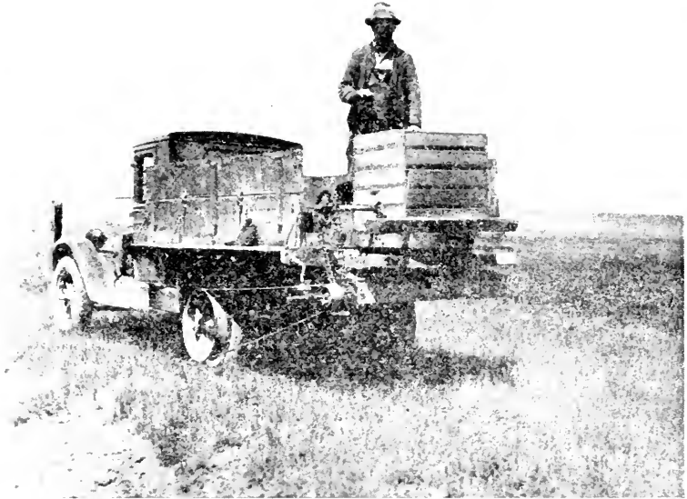
Figure 4.—A mechanical grasshopper-bait spreader mounted on a truck and operated by belt from rear wheel.
