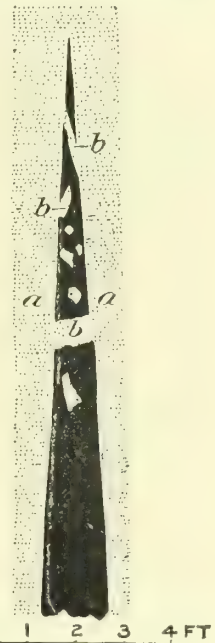
FIG. 31.—Terminal cross section at outcrop of Black Dragon vein, Evacuation Creek. aa , Country. bb , Fragments of wall rock.
