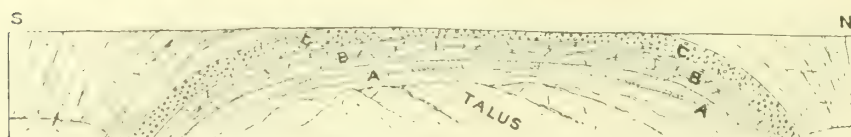
FIG. 37.—Sketch showing fold in brick-clay beds and associated gravels on the western side of Fresh Pond, Cambridge, Mass. From a sketch by J. B. Woodworth made in 1891. A, Fine sands, cross-bedded, with a few layers of clay; B, gray clay, similar to brick clays, with minute faults and joints, 10 feet; C, waterworn pebbles in coarse gravels.
