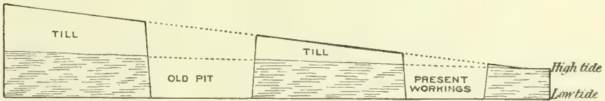
FIG. 43.—Section showing relations of till to brick clays in East Saugus, Mass.
