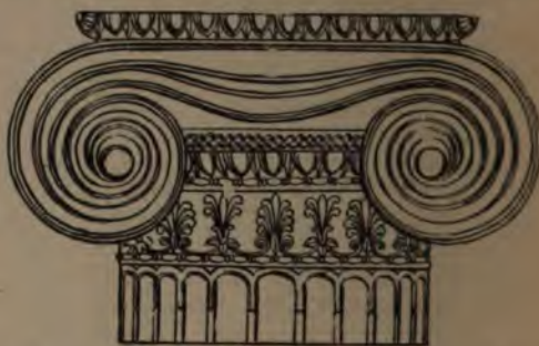
FIG. 1.—IONIC CAPITAL OF THE EASTERN PORTICO OF THE ERECTHEIUM.
