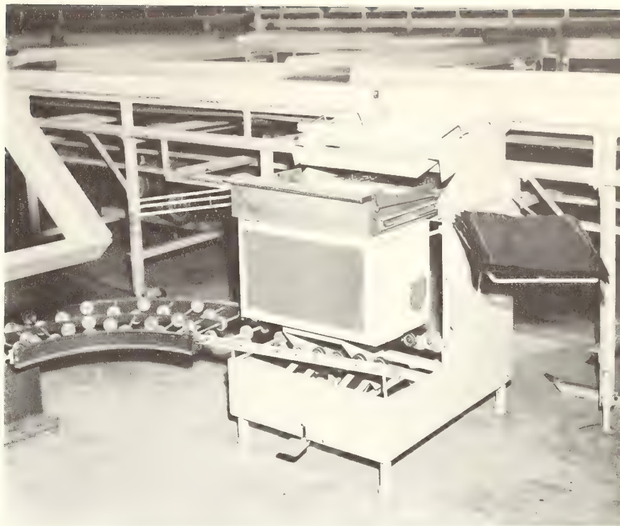
Figure 3.--A semiauto- matic tray-packing machine.
