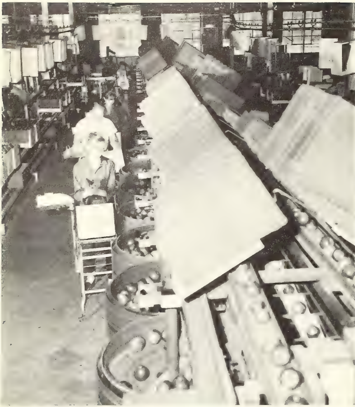
Figure 1.--A typical packing line using rotating tubs.
