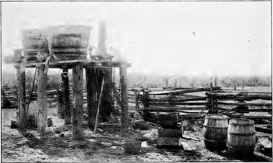
FIG. 35.—A good equipment for making lime and sulfur. The engine pumps water from a pool at left, and the boiler furnishes steam for cooking the mixture
