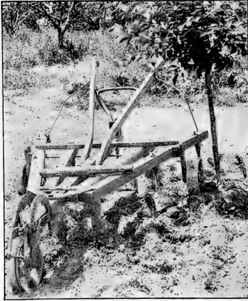
FIG. 33.—A poor type of cultivator for orchard use. Both frame and handles "skin" many trees
