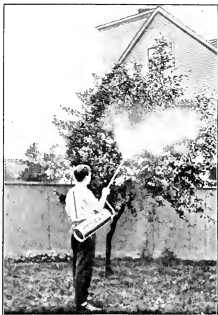
FIG. 113. A small compressed-air sprayer Practical for the home gardener or for very young trees
