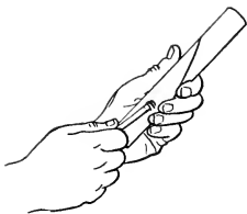
FIG. 33. Punch hole in side of cartridge with round, pointed handle of cap crimper
