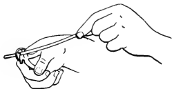
FIG. 35. Crimp the blasting cap to fuse securely with Du Pont cap crimper
