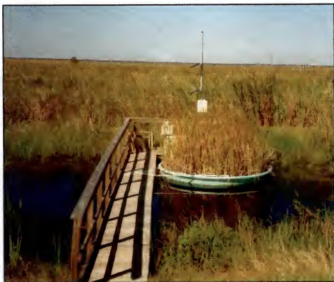
Figure B.1 Cattail lysimeter in the Fort Drum marsh.
