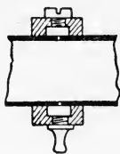
FIG. 709.—Section of pressure gauge connection.
